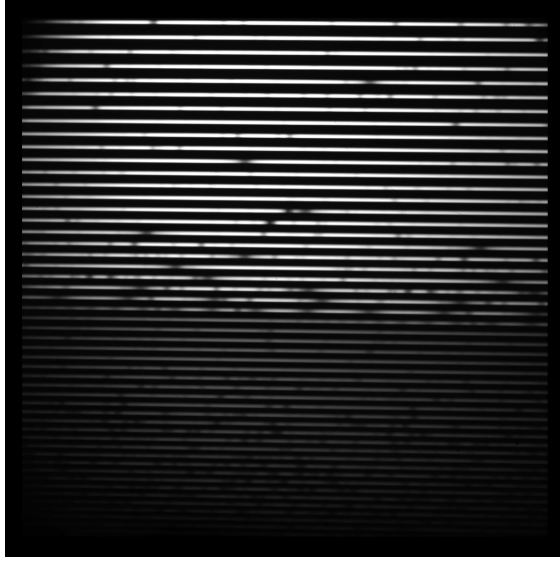
(a) Echelle spectrum image obtained with the NES spectrograph
