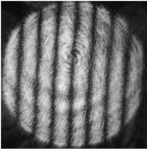
Fig. 9. Interferogram of the Ø50 mm modulator wavefront with applied voltage.
