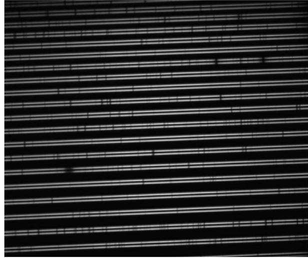
**Fig. 4.** An image of the  $\beta$  Aql (G8 IV) spectrum on-screen when using the diffraction grid as a cross-dispersor. The red region is at the bottom. The spectrum is derived with an analyzer of circularly polarized light, therefore each order is divided into two spectra. The strong line is in the lower part of the image –  $H_{\alpha}$ . The sodium doublet is well seen in the top right corner
